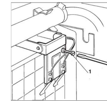
The ice thickness probe can be adjusted for thicker or thinner ice cubes by screwing the adjusting screw (1) clockwise for thicker ice or for thinner ice counter-clockwise. **NOTE:** Ensure the ice cubes have a 3mm concave dimple on the back of the cube. The ice bridge connecting the ice cubes should be between 2mm and 3mm thick. Never turn the adjusting screw more than  $\frac{1}{4}$  of a turn at time.
