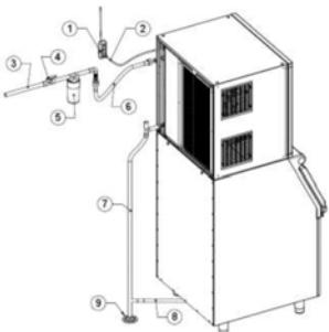
Fit the water supply hose and the water drain hose to their connection points at the rear of the ice maker using hoses supplied. Connect the water supply hose to the water filter outlet, attach the water drain hose to the floor drain or tundish.
