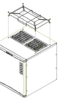
Fit the steel deflector plate to (back right side) of the ice maker. This is to prevent recirculation of hot air back into the ice maker. **(On the NW307/507 models fit the wire frame to the top of the machine to prevent the discharge vents being covered)**
