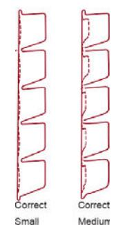
The ice thickness probe can be adjusted for thicker or thinner ice cubes. By carefully loosening the ice thickness float bracket screw, move the bracket up slightly (**for thinner ice**) or down slightly (**for thicker ice**). Take a photo of the bracket position before you make the adjustment. Only move the bracket 1mm at a time, check the ice thickness after the two drops of ice after the adjustment has been made.
