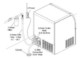
Maneuver the machine into its final position. **Ensure the ice machine has required 150mm side clearance and 100mm rear clearance.** Ensure the machine is level once in its final position. Remove the protective plastic from the panels of the machine and ice storage unit.
