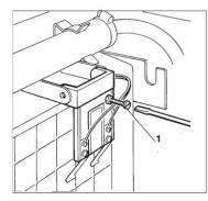
The ice thickness probe can be adjusted for thicker or thinner ice cubes by screwing the adjusting screw (1) clockwise for thicker ice or for thinner ice counterclockwise. NOTE: Ensure the ice cubes have a 3mm concave dimple on the back of the cube. The ice bridge connecting the ice cubes should be between 2mm and 3mm thick. Never turn the adjusting screw more than ½ of a turn at time.
