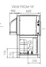
UNIT OF MEASUREMENT: **mm** 1. 13/16" OD - OVERFLOW DRAIN 2. 3/4" GAS - WATER INLET 3. 3/4" GAS - WATER OUTLET WATER COOLED UNIT ONLY
